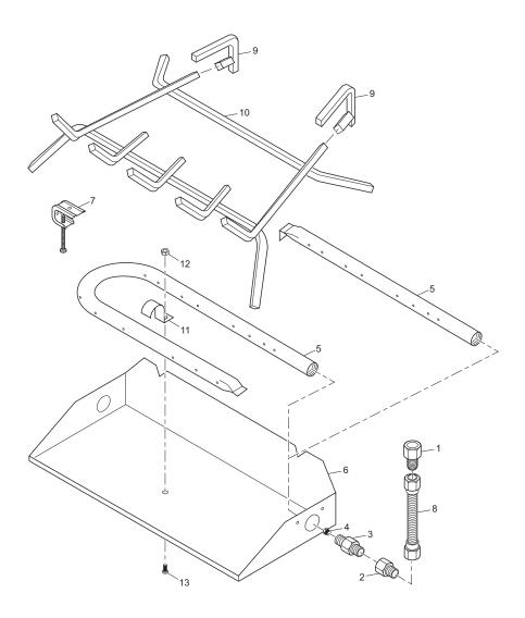
This list contains replaceable parts used in your log set. When ordering parts, follow the instructions listed under <u>*Replacement Parts*</u> on page 19 of this manual.
